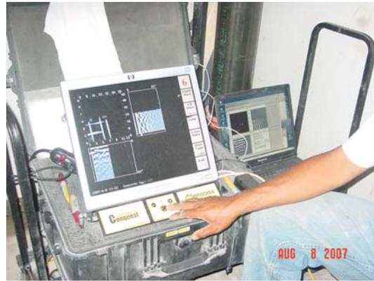
Scanning for existing reinforcing bar – slab penetration submittal process
